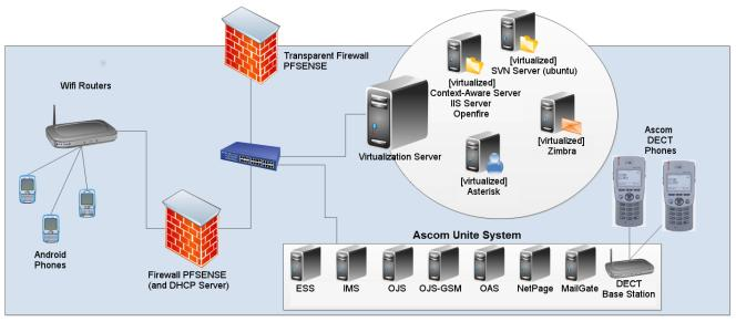
Figure 2: CallMeSmart prototype network structure
