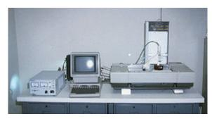
Fig. 1: Early version of a 3D printer
