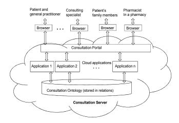
Figure 2. The components of the cloud-based Consultation Server.
