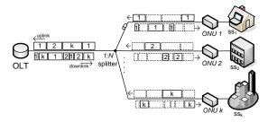
Figure 1. EPON system: upstream (multi-point to point) and downstream (point to multi-point) transmission.
