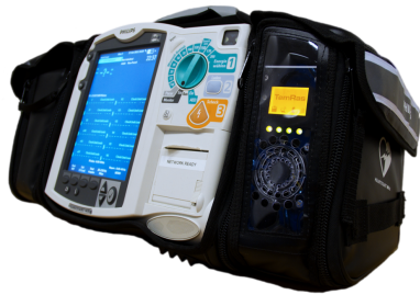
Figure 3. An early development prototype of the on-scene peeqBOX fitted inside the right pocket of the monitor/defibrillator-device's bag. The bag's right pocket was later adjust to provide space for patient therapy equipment.
