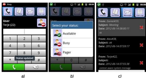
Figure 2: a) CallMeSmart SoftPhone keypad, b) The dialog box from which the user can switch the phone's operating mode manually, c) the Message List
