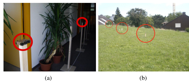
Fig. 5. Indoor (a) deployments using IRIS motes and outdoor (b) deployments using AVRRAVEN motes.
