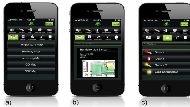
Figure 4. iPhone Prototypes. a) Choice of different maps. b) Map view of humidity gradient. c) Display of notifications.
