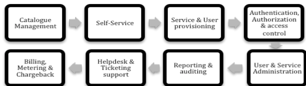
Figure 6: Workflow of a CSB Platform [13]
