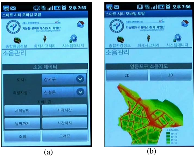
Figure 3. Snapshots of the Environment Information Manager of UTOPIA in a smartphone : (a) A Noise Monitoring, (b) A 2D/3D Noise Map.
