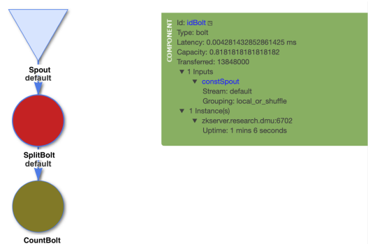
Figure 9. Congestion caused by high input data rates and its effects on the processing capacities of the various topology components.
