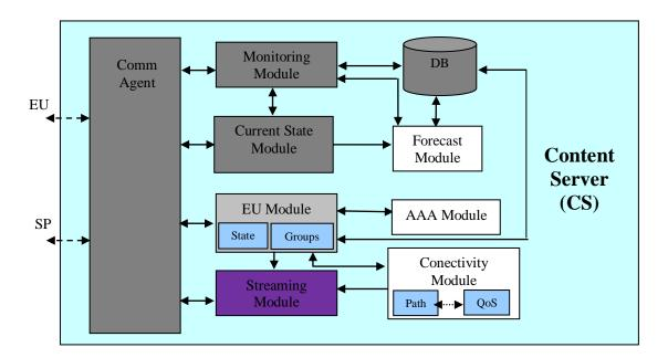
Figure 4. The Content Server software architecture
