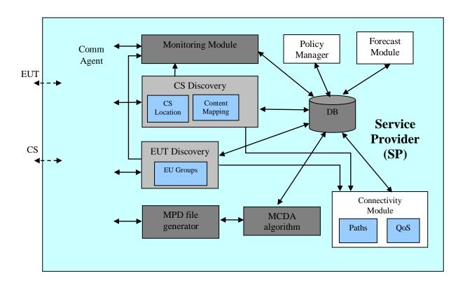
Figure 2. The Service Provider software architecture
