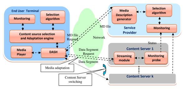
Figure 1. DISEDAN general architecture; DASH - Dynamic Adaptive Streaming over HTTP
