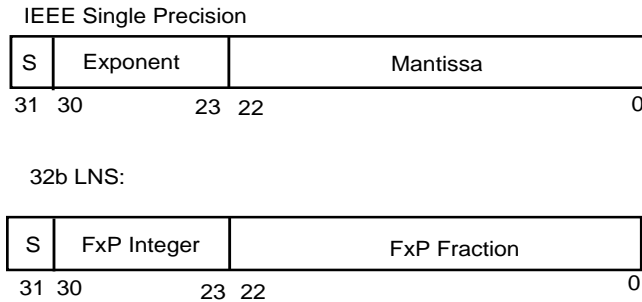
Fig. 1. IEEE standard single precision floating point representation and the 32-bit LNS format.
