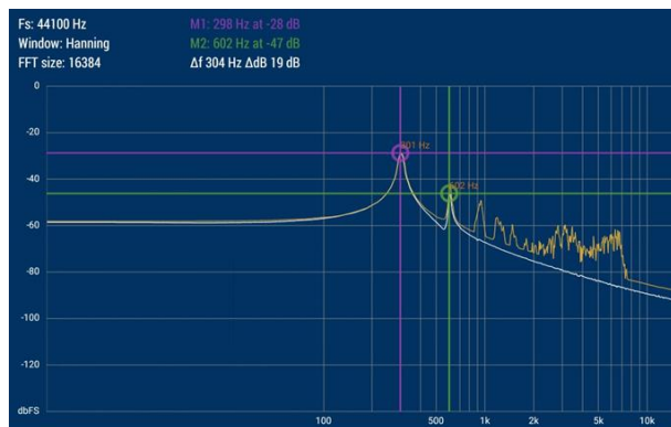
Figure 9. Fundamental frequency measure on Rijke tube experiment.
