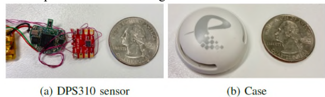
Figure 2. The proposed fall detection sensor node, which consists of a a BSN node, a battery, and a casing of the sensor (with a quarter US dollar coin on the side)
