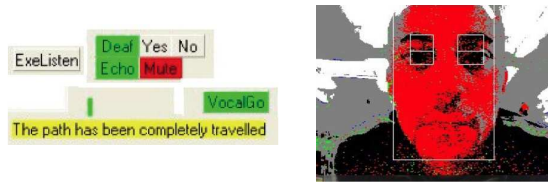
Figure 17. On the left, Piaget panels and text-typed fields illustrate typical vocal dialogues: e.g., recognized commands are shown in green (here “”) and synthesized text in yellow; yes/no buttons can at will simulate microphone inputs. On the right a face is recognized for “Who is Who” test.
