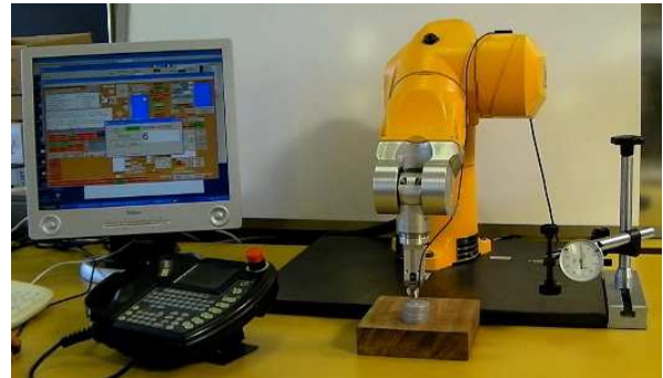
Figure 20. “Chip count and accuracy test”: Application mostly developed and programmed in Piaget, including the industrial robot arm visible on the picture and other resources: optical fiber, PLC, camera, motorized rotating table, servocontroller, Ethernet switch, PC and other components yet.
