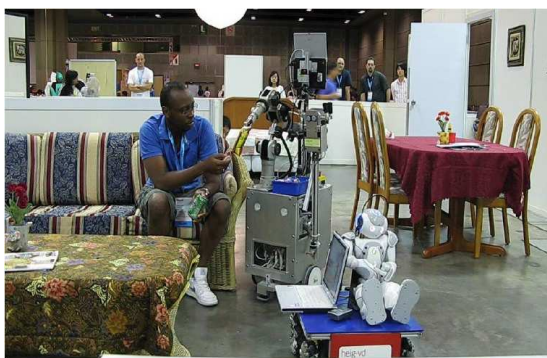
Figure 19. “Open Challenge” (Robocup@Home world competition, Singapore). Nono, a NAO-typed robot, discusses with “Daniel”, moves on OP-Y platform and then calls RH-Y, which brings drinks and snacks. Application developed and programmed in Piaget
