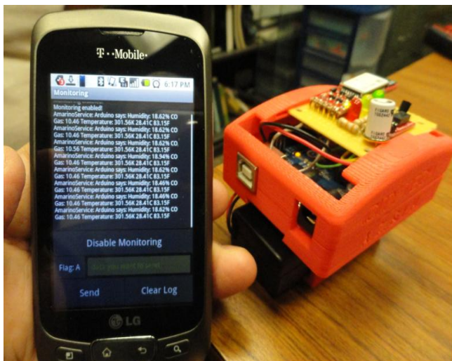
Figure 15. Indoor Testing Using Smartphone.
