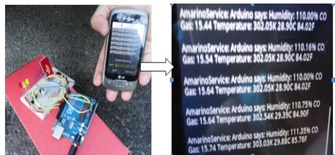
Figure 19. Outdoor Testing Using Smartphone.
